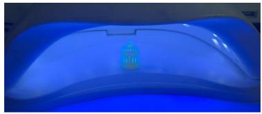
Step 13: Irradiate the model with UV-light about 2-3 mins.
