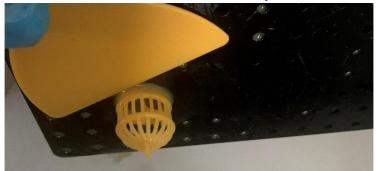
Step 11: Remove the model from the platform.
