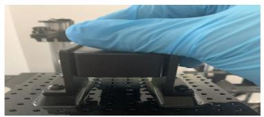
Step10: Loosen the handle and remove the platform.
